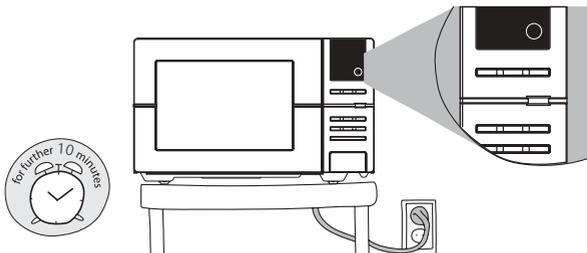
**4** Ten minutes after cooking is finished the oven will automatically go into Zero Standby and use no power.
