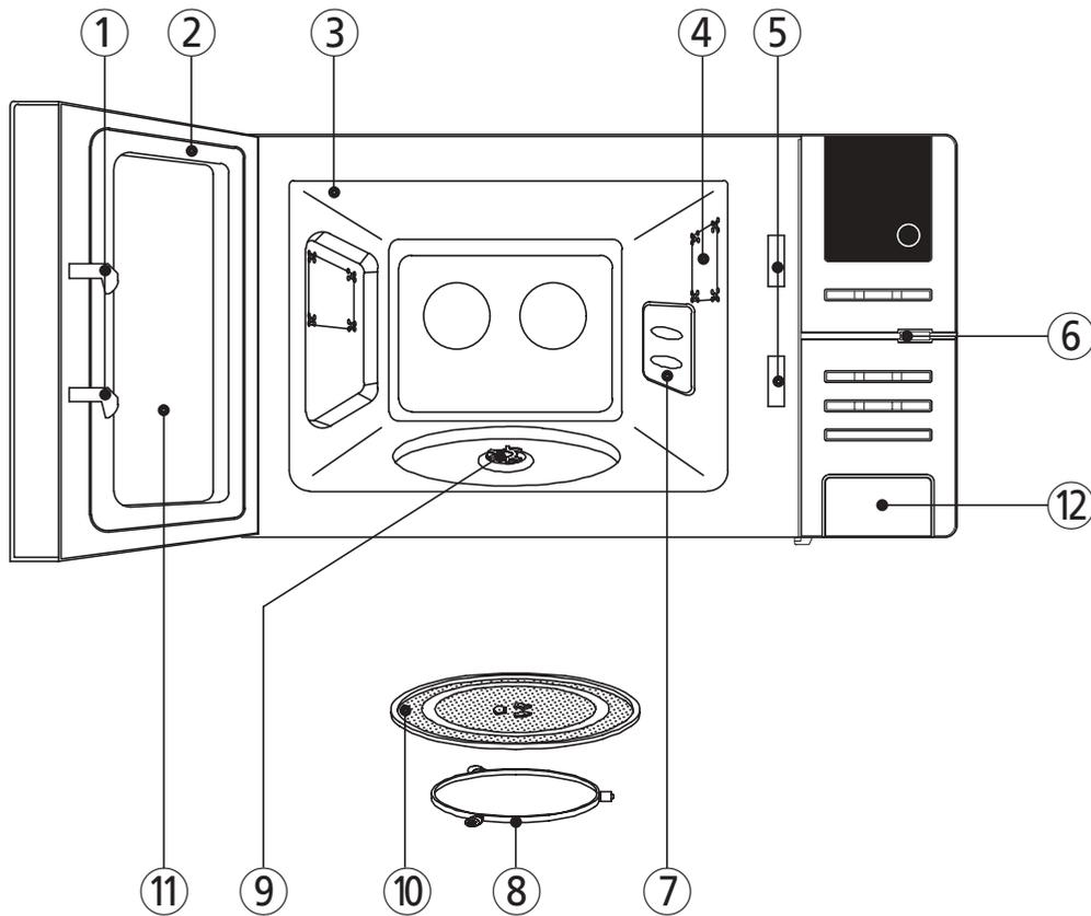
① **Door latch** - When the door is closed, it will automatically shut off. If the door is opened while the oven is operating, the magnetron will automatically shut off.
