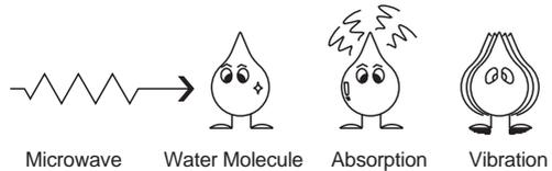
The microwaves cause the water molecules to vibrate which causes **FRICITION**, i.e. **HEAT**. This heat then cooks the food. Microwaves are also attracted to fat and sugar particles, and foods high in these will cook more quickly. Microwaves can only penetrate to a depth of 4-5cm and as heat spreads through the food by conduction, just as in a traditional oven, the food cooks from the outside inwards.
